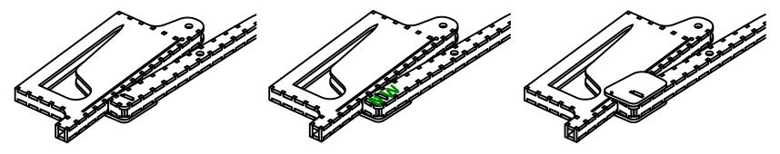
C) Add glue as shown in green, then glue down the other stock cheek, pointy end in the bolt box slot. Let dry.
