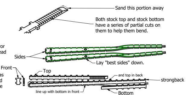
D) Not shown. Wind rubber bands tightly around entire assembly to clamp while the glue dries. The rubber bands should force the top and bottom to bend to the same curvature as the stock.
